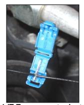
Figure 4 (T-Tap connector installation)
