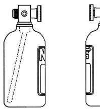
Figure 2 Nitrous Bottle Siphon Tube Orientation
