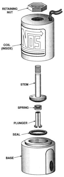
**Exploded View of a Typical Solenoid**
