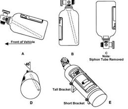
Figure 3 Nitrous Bottle Mounting Orientations
