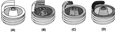
**Figure 13 Spark Plug Condition**
