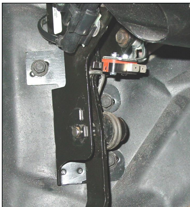
Figure 16 Microswitch in completed location
