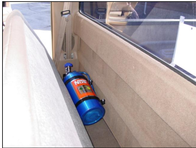
Figure 4 Bottle with blow down tube installed
