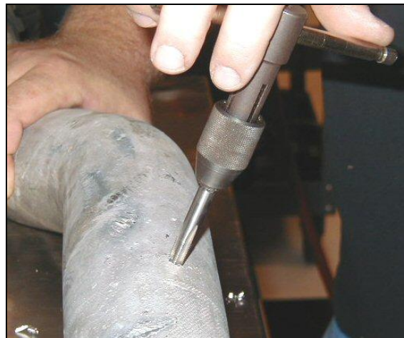
Figure 7 Tap with supplied 1/16 NPT tap.
