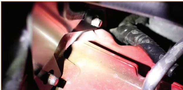
15. Install the Mishimoto hose with the 90° bend to the port marked **IN** on the catch can. This is the hose that comes from the valve cover. Secure the hose with the worm-gear clamp. (1x worm-gear clamp)
