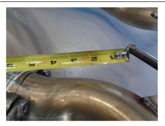
**Step 2.** Begin removing the OEM exhaust system by cutting both pipes exiting the resonator. Measure and cut on the driver side 5" from the tip of the hanger. Cut the passenger side also from the tip of the hanger 5.5" back. Next, extract the hangers from the rubber insulators and remove the OEM mufflers. Retain insulators as they will be used to install the new system.
