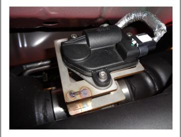
**Step 5.** If your vehicle has valves, re-connect the wiring harness plugs to the Valve motors and wire mounting bracket.
