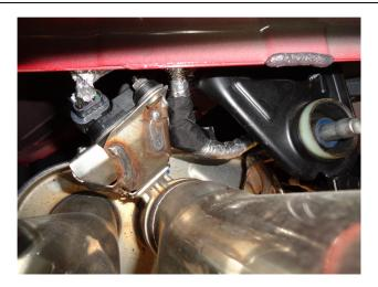
**Step 1.** To begin, determine if your vehicle has OE exhaust valves, if so, you will need to unplug and the electrical connection on the Exhaust Valve Control Motors (Qty 2)located on the OEM exhaust assembly, also disconnect wire harness mounting plug.
