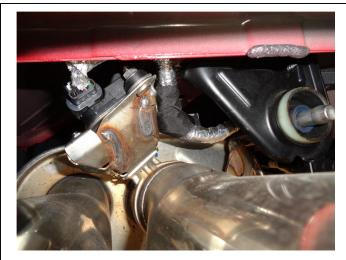
**Step 1.** To begin, determine if your vehicle has OE exhaust valves, if so, you will need to unplug and the electrical connection on the Exhaust Valve Control Motors (Qty 2)located on the OEM exhaust assembly, also disconnect wire harness mounting plug.
