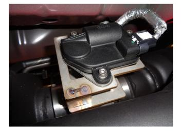
**Step 6**. If your vehicle has valves, re-connect the wiring harness plugs to the Valve motors and wire mounting bracket.
