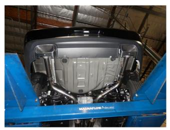
**Step 5.** Once the tips are removed install the OEM Tailpipe extensions using 2.50" Supplied clamps and fit into rubber insulators. Finish by installing the Stock tips to these extension pipes using the supplied ball clamp.
