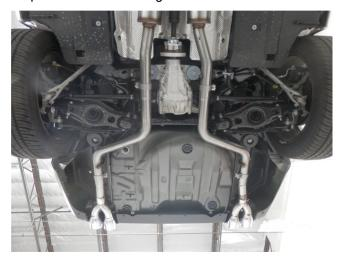
**Step 3.** Attach the Mid-pipes to the Resonator Assembly with supplied 2.50 Clamps and fit hangers into rubber insulators. RemeMber to re-attach the ground strap to the hanger. At this point you have two options for tips. Magnaflow supplies a Quad tip setup that can be clamped to the Mid-Pipes and held in place with hangers and the installation is complete.
