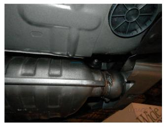
**Step 4.** To install the OEM tips they must first be removed from the stock exhaust system. You will need to loosen the tip clamps and break the weld holding them to the mufflers, both sides.
