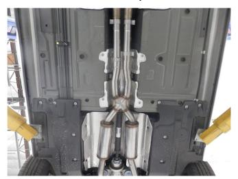
**Step 2.** Begin installing of the new system by attaching the Driver and Passenger side (Passenger is the longer of the two pipes) inlet pipes to the outlets of the OEM system using the supplied 2.50" clamps. Next attach the Resonator Assembly to the inlet pipes with supplied clamps and insert the hangers into the rubber insulators.
