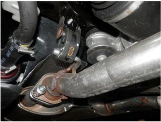
**Step 1.** To begin the removal of the OEM system you will need to unfasten the X-Pipe inlets at factory clamp locations. Next un-clip the ground strap from the passenger side muffler hanger. Working rearward (with the exhaust supported) extract the hangers from the rubber insulators and remove the OEM exhaust. Do not discard or damage the rubber insulators as they will be used to install the new exhaust system.
