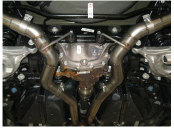
**Step 2.** Begin installation of the new system by attaching both Inlet Pipe Assemblies to the pipes you have just cut. Loosely secure using the supplied 2.50" clamps. Engage the welded hangers to the rubber insulators. Leave all clamps loose until final adjustment.
