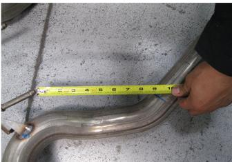
**Step 1.** Begin removing the OEM exhaust system by cutting both pipes going into the muffler assemblies. Measure and cut 9" forward of the welded hangers as shown. Next working front to rear extract the hangers from the rubber insulators and remove the OEM system. Retain insulators and clamps as they will be used to install the new system.
