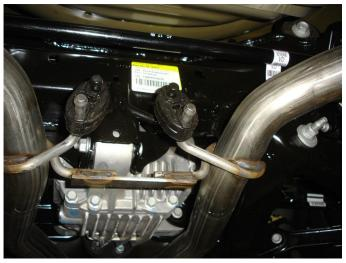
**Step 2.** To remove the OEM exhaust loosen the two bolt clamps located behind the catalytic converters. Working rearward disengage the rubber inulators from the welded hangers, retain clamps and rubber insultors as they will be used to install the new system. Remove complete system.
