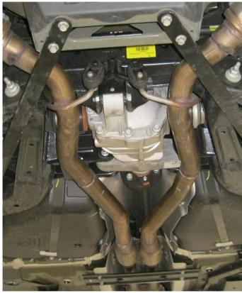
**Step 1.** Begin by removing the two front crossmembers and the two rear chassis stiffeners by the muffler inlets. This will allow access to the exhaust system.
