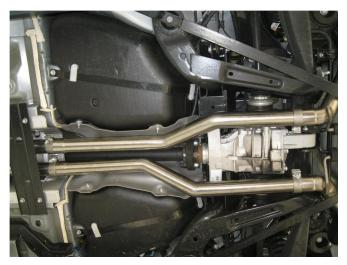
**Step 4.** Next, attach the Driver and Passenger Side Extension Pipes (as shown) to the Resonator Assembly using the supplied 2.50" clamps.
