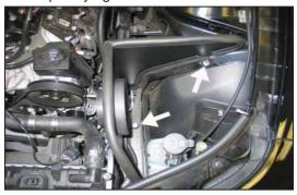
15. Install the heat shield assembly into the vehicle so the inserted nut goes into the airbox mounting grommet hole and the tab goes onto the airbox mounting stud. Secure the heat shield with the provided hardware.
