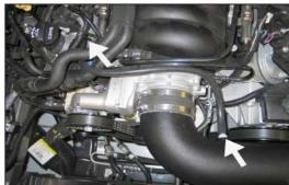
24. Attach the provided crankcase vent hose to the 1/4" NPT fitting and then attach the open end to the vent port on the valve cover.
