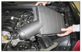
9. Lift up and remove the airbox from the vehicle. NOTE: K&N Engineering, Inc., recommends that customers do not discard factory air intake.
