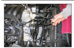
7. Rotate the crankcase vent tube 180°, then release the retainer at the valve cover port and then remove the crankcase vent tube from the valve cover port.
