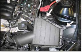
8. Remove the two airbox retaining nuts shown.
