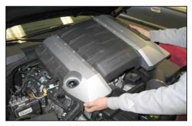
3. Remove the oil filler cap and then lift up and remove the engine cover. Reinstall the oil filler cap.
