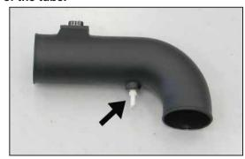
22. Install the provided 1/4 NPT fitting into the  $K\&N^{\odot}$  intake tube as shown.
