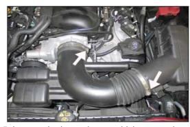
5. Loosen the hose clamps which secure the stock intake tube to the airbox and throttle body.
