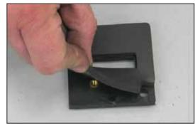
19. Install the provided gasket onto the mass air sensor adapter as shown.
