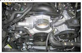
16. Install the silicone hose (08761) onto the throttle body and secure with the provided hose clamp.
