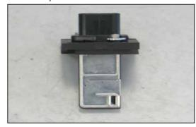
20. Install the mass air sensor into the adapter and secure with the provided hardware.
