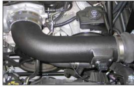
23. Install the K&N® intake tube assembly into the silicone hose at the filter adapter and then into the silicone hose at the throttle body and secure with the provided hose clamps.
