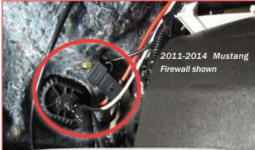
Route the thick Red, White wires and the Silver/Brown Control Wires through the modified firewall bulkhead grommet. To modify the grommet: Remove the Inner Fender Liner, use a razor blade to cut the nipple that sticks out of the grommet.
