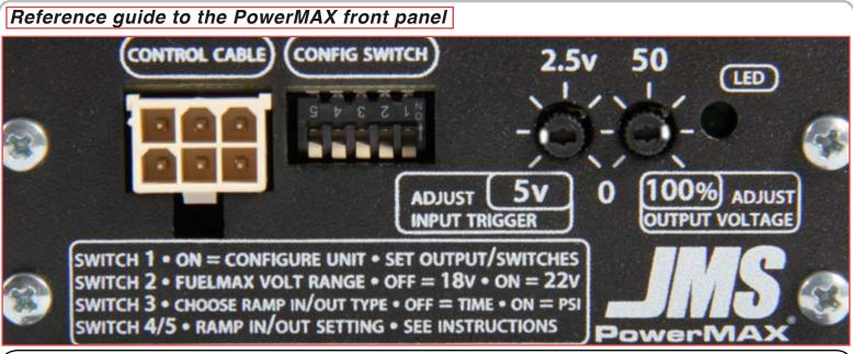
Set Dip Switch 1 ON to ADJUST boosted output voltage: Set via Adjust Output Voltage Knob. Adjust Output Voltage: 0 = 14.5v boosted output; 100% = 25v or 31v boosted output (depending on the range: dip switch 2)
