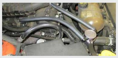
Remove factory PCV hose then install Oil Separator Kit as shown in picture. Making sure the shorter hose goes to intake manifold/draw side.
