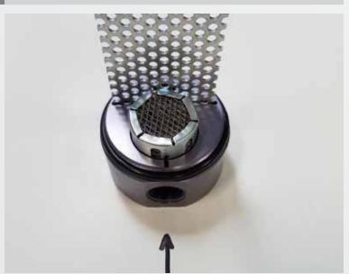
This picture (Note) As the arrow shows this is the draw side of the oil separator. The hose that goes to the intake manifold will attach to this end.
