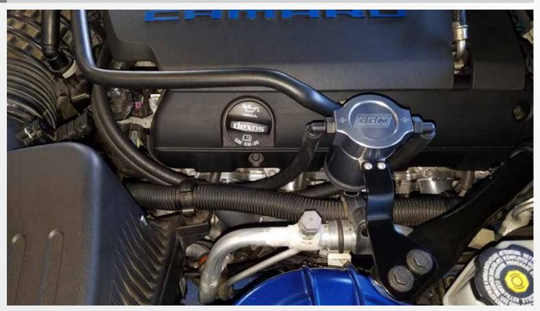
Remove factory strut tower bracket bolts then mount oil separator assembly, then run hoses forward and use supplied clamps at engine connection. Use 1/4 socket and ratchet to tighten clamps do not over tighten then use supplied zip tie for loose hoses as shown in picture.
