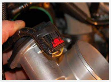
Remove the four mounting bolts from the stock throttle body, as you remove the throttle body flip it to unplug the motor plug on the bottom.
