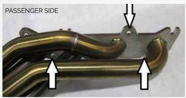
Using an 8mm Torx bit socket remove all the exhaust studs. Only leaving the (3) studs that correspond to the marked holes pictured below. (This will be done to the driver side and passenger side of the engine.) The supplied bolts will be used in the holes that the exhaust studs where removed.
