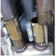
On the 2015 model loosen the ball flare clamp on the driver side pipe near the transmission cross member then loosen the exhaust coupler at the resonator and remove driver side pipe from the vehicle.
