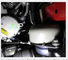
NOTE: Remove the 2 bolts that hold the actual motor mount isolator to the chassis as the entire motor mount assembly needs to be removed on the passenger side to allow room to install the BBK Header on all years from 2011 to 2015
