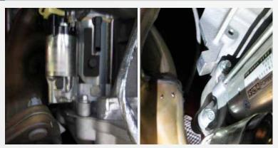
Remove the (3) 10mm bolts that hold the starter in place then remove the starter and hang it to the side.
