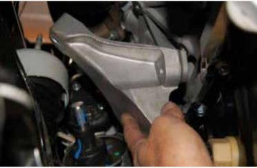
Utilizing a jacking device and a block of wood under the bell housing, remove the previously loosened nut on the driver side motor mount, once removed jack the engine upward enough to clear the motor mount stud. Remove the 4 bolts that secure the aluminum mount to the engine block and remove from the vehicle.
