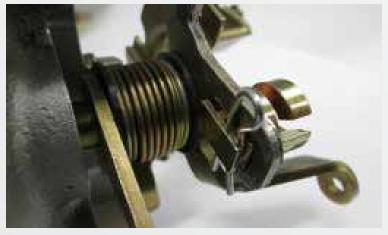
NOTE: On Ford Ranger only Install the throttle cable adapter with the open slot end facing down and install the safety clip onto the back side of the adapter.
