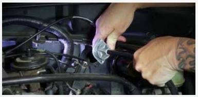
Working from under the hood, remove the sheetmetal screw attaching the clutch cable housing to the firewall. Once removed, simply pull the housing and exposed cable from the opening in the firewall.
