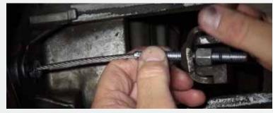
Reattach the cable to the quadrant assembly first, then to the clutch fork. To adjust the cable, simply twist the knurled adjuster either cw or ccw to loosen or tighten cable.
