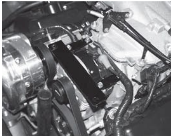
Scoop Support Installed
