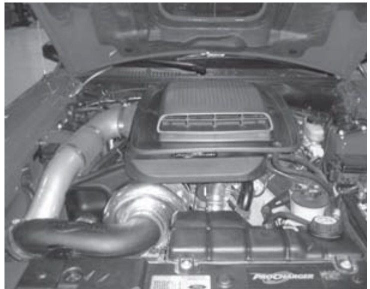
System Installation with Shaker Interface Duct
