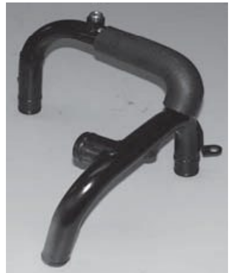
Coolant Manifold Assembly
