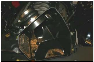
7. Transfer the factory air box mounting grommets. A) 8. Install the hump hose (#5) onto the filter adapter using
