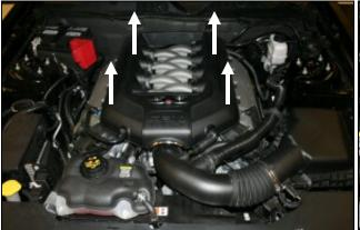
**Disconnect The Negative Battery Terminal!** 1. Remove the Engine cover by simply lifting up, and set aside.
