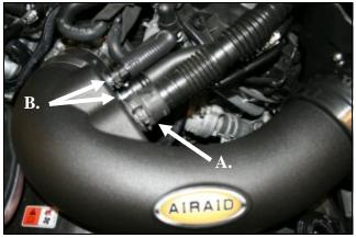
11. Install the Airaid Intake Tube into the couplers as 12. A) Install the Airaid Premium Filter (#1) onto the shown, and tighten all Hose clamps. A) Reconnect the filter adapter and tighten the hose clamp. B) re install the Resonator tube to the Airaid Intake using the OEM Resonator tubing into the factory Stand off. clamp. B) Reconnect the breather line/lines to the Aluminum Fittings depending on your application.
