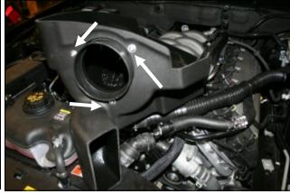
head bolts (#10), and flat washers (#11) into the Airaid Cool Air Box (CAB) (#4) as shown.
