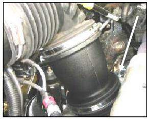
7. Install the Airaid Intake Tube assembly onto the turbocharger inlet. Tighten the factory hose clamp.
