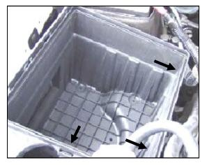
3. Unlatch the three clips on the factory air box. Remove the factory intake tube assembly and airbox lid from the vehicle.
