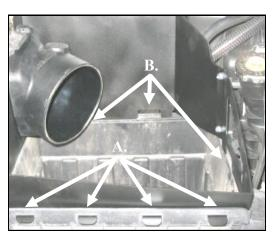
11. A.) Install the CAD by inserting the four tabs into the side of the factory airbox.B.) Relatch the three airbox clips onto the CAD.
