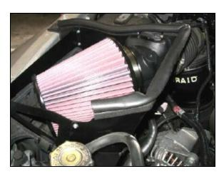
**14.** Install the Airaid Premium Filter (#1) onto the air filter adapter, and tighten the clamp. Install the weather strip (#6) onto the top of the **CAD.** (Hint: start at one end, and work to the other).
