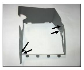
8. Assemble the Airaid Cool Air Dam (CAD) panels (#2, #3) using four 6-32x 5/16" screws (#7), #6 flat washers (#8) and 6-32 keps nuts (#9).
