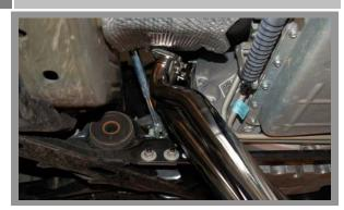
Install the BBK Full Length Headers from underneath the vehicle. They will slip right in place and onto the studs. Install all the nuts and tighten both sides.
