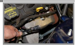
Remove the strut tower brace if equipped.
