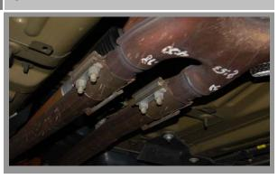
Loosen the 2 nuts on each of the barrel style clamps that connect the exhaust system to the stock X-Pipe. Remove the nuts at the exhaust manifold collectors and remove the entire X-Pipe assembly. From the top of the engine compartment, remove the stock nuts that bolt up the stock exhaust manifolds and remove from vehicle along with the stock gaskets.
