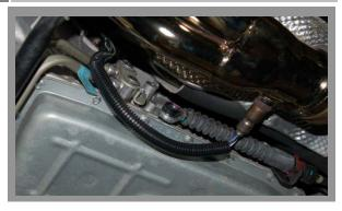
Remove the front oxygen sensors from the stock cat back pipe and install them into the BBK Full Length Header Collectors. Route the driver side oxygen sensor wires under the shift lever and zip tie to one of the steel Transmission cooler lines. <u>NOTE!!!</u> Be sure to add a small amount of anti-seize to the top thread of each oxygen sensor using the supplied anti-seize packet. As you thread the oxygen sensor back into the part the antiseize will spread evenly throughout the threads.
