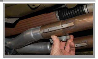
Install the provided studs into the collector flanges of the BBK Headers. Install the BBK X-Pipe kit.
